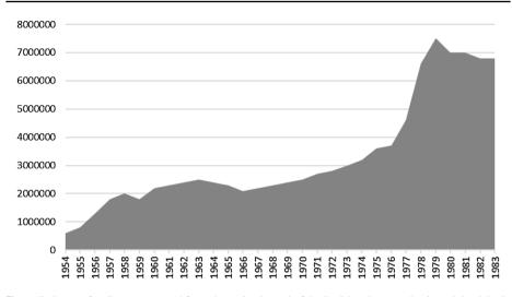
Fig. 3 Estimate of sediment extracted from the main channel of the Po River between Pavia and the delta in m3/year. Chart by the authors with data from Lamberti et al. 1990, pp.195–196
